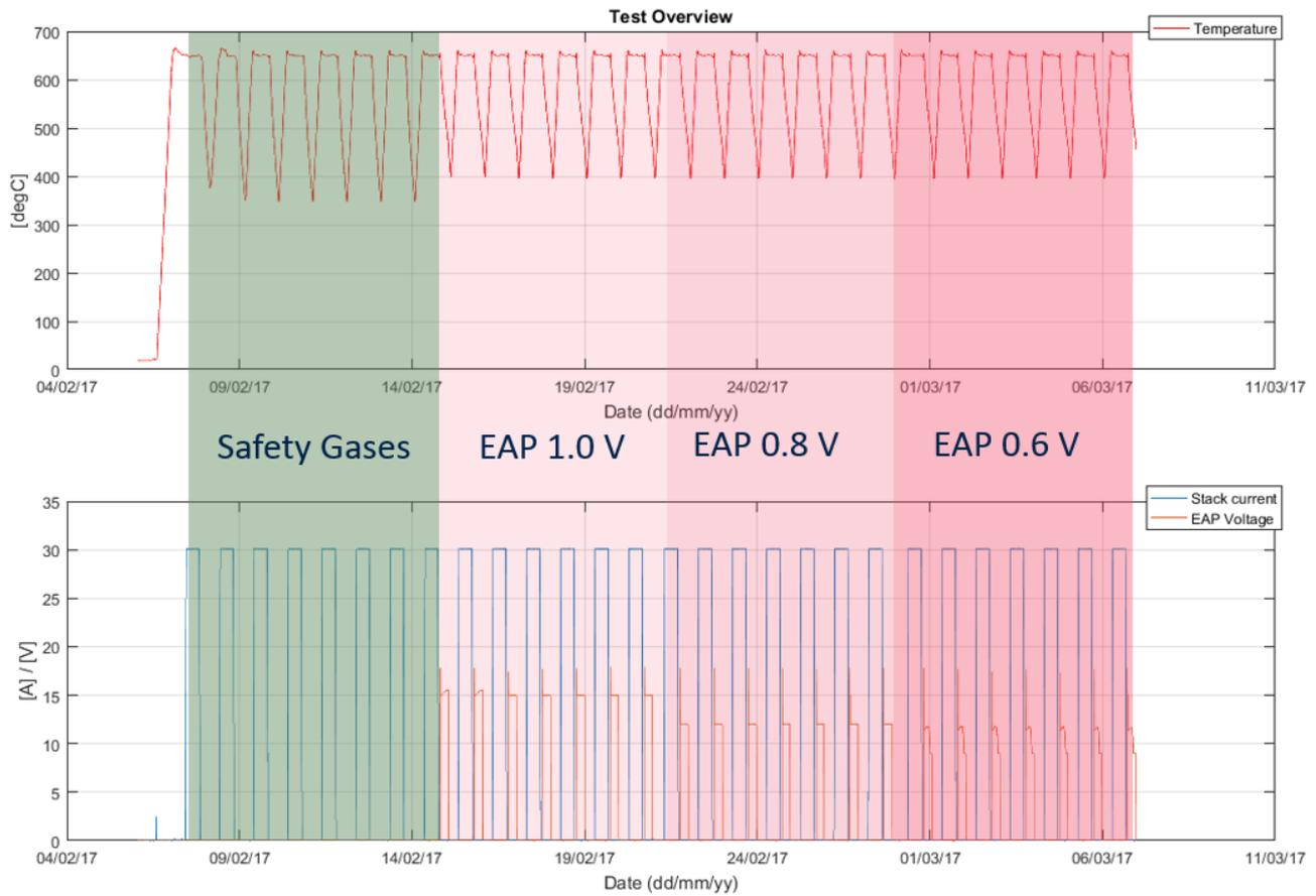
Figure 5. Overview of conducted test run. Temperature, stack current and EAP Voltage curves are shown.
