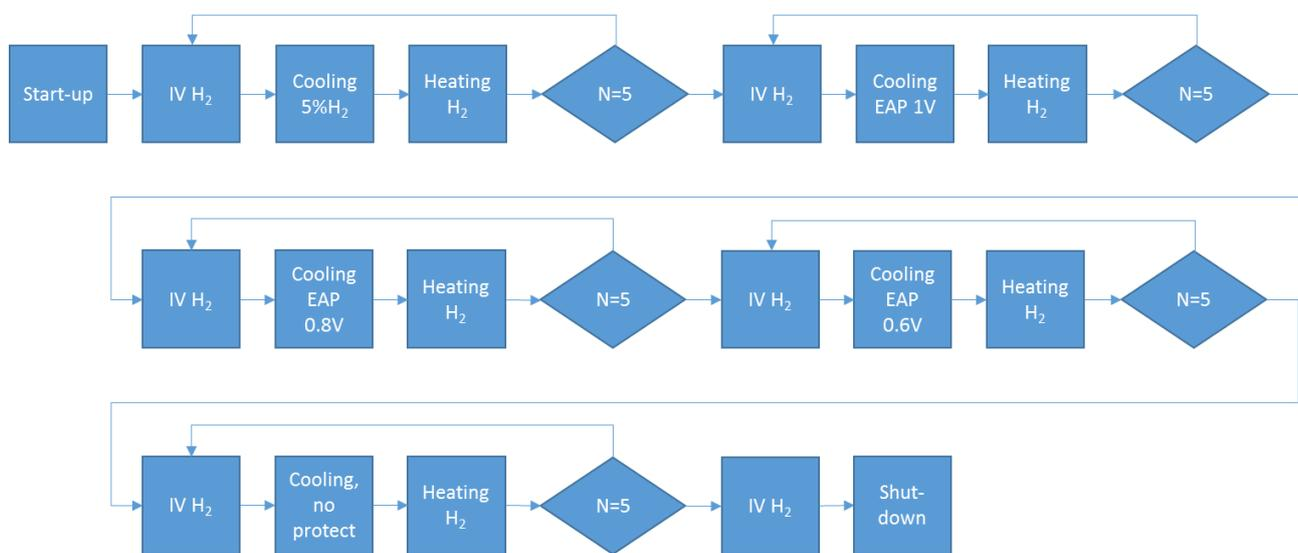
Figure 4. Initial test plan for EMSD test (cycles was changed from N=5 to N=7)
