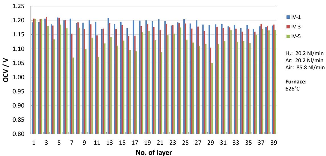
Figure 8. Comparison of the OCVs at ~15 h, 1430 h and 2300 h
