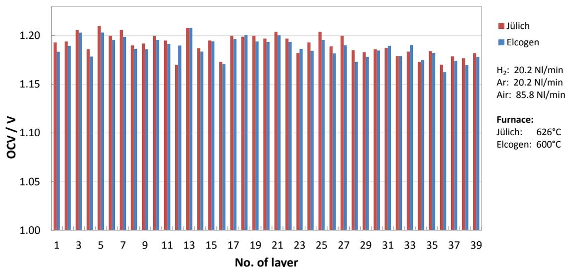
Figure 2. Comparison of the OCVs of stack 300017030601 measured at Jülich and Elcogen
