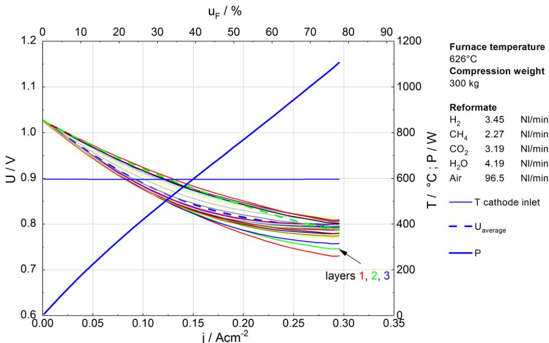
Figure 3. Performance of the stack 300017030601 with simulated reformat measured at Jülich
