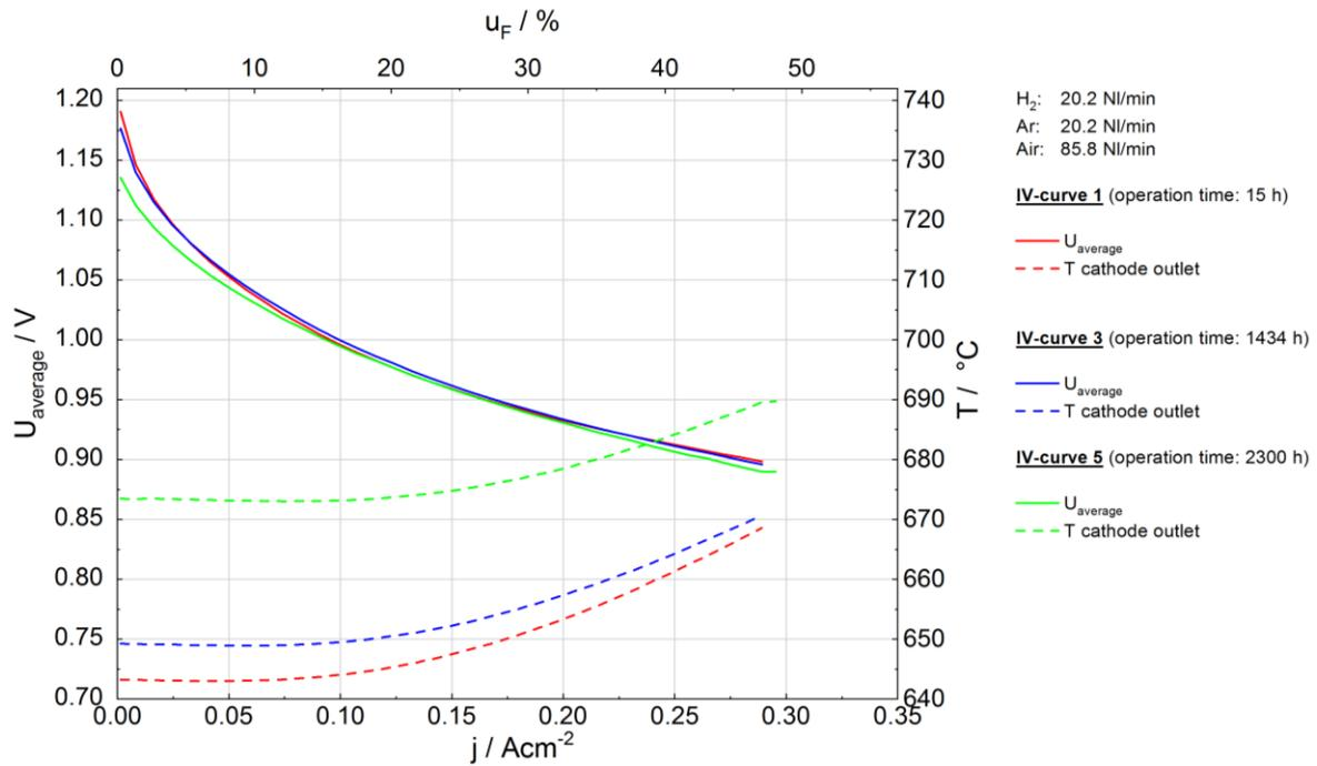
Figure 7. Comparison of the I-V curves at ~15 h, 1430 h and 2300 h
