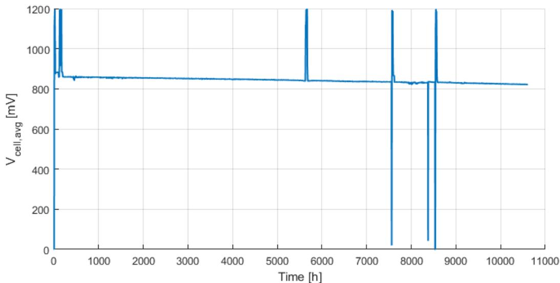
Figure 9. Elcogen stack, average cell voltage in the long-term test.
