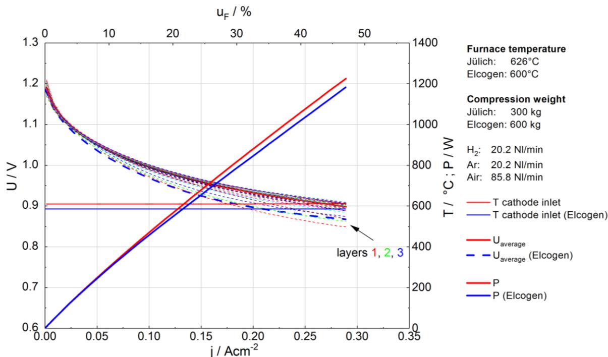
Figure 1. Comparison of the performance of stack 300017030601 measured at Jülich and Elcogen
